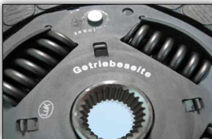
Images 1-4: Possible markings on the clutch disc
